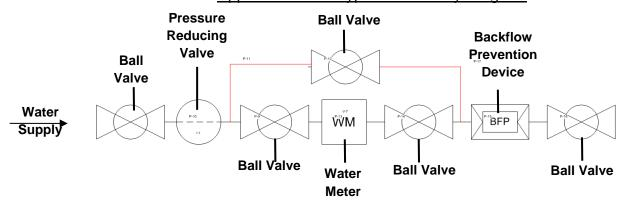
All Water Service installations must conform to the current Rules and Regulations. The above diagrams are the current approved metering system assemblies. District notification is required to operate the bypass.
