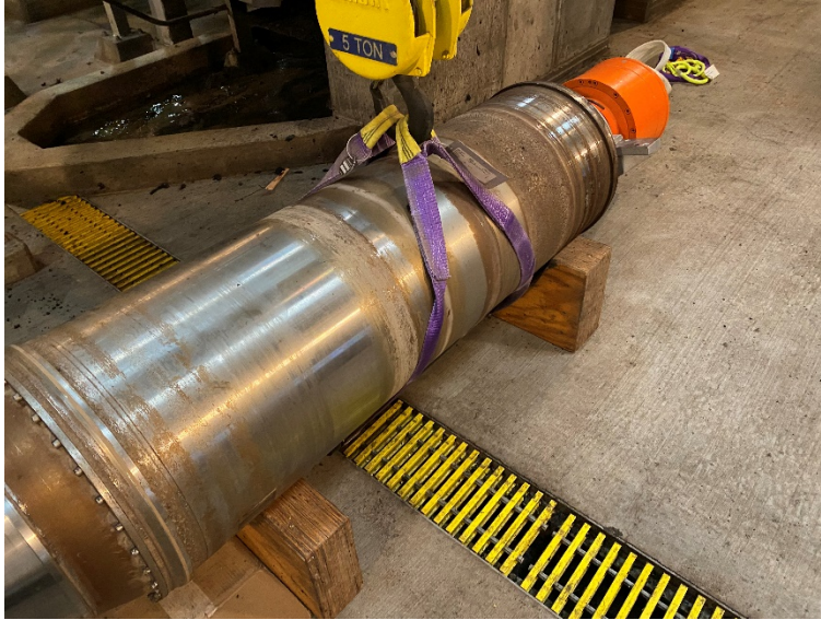
Rotating components of the Edwards WW west centrifuge unit were removed, and bearings were replaced.
